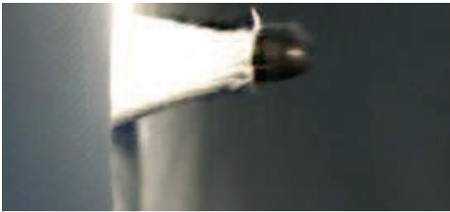
Figure 3: Elongation of knit fabric increases bullet-to-fabric contact (high speed image)
